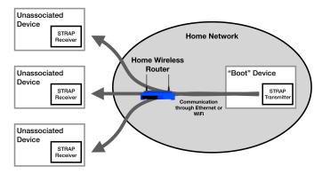
Fig. 1: Overview of STRAP components. The boot device securely sends the network name and password out of the home network to the unassociated devices.
