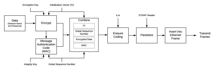
Fig. 4: Flow of data through STRAP
