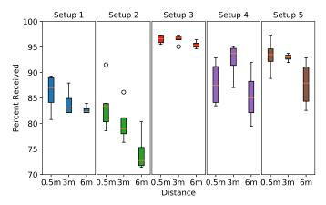
Fig. 5: Percent of frames received in different experimental setups (different wireless routers, different locations) vs. path length.
